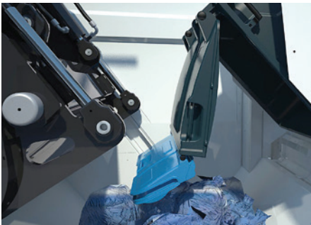
Contact with waste in the loading hopper
